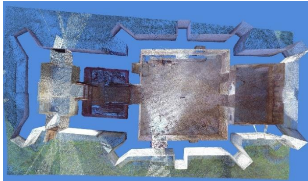
Figure 7. The projection of the church at the level of the sanctuary +1.0m, obtained with ReCap software
