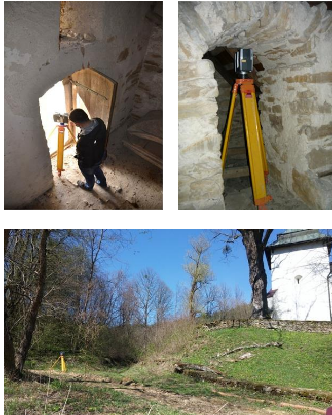
Figure 2. TLS measurements: - indoor and outdoor measurements
