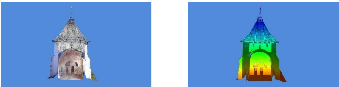
Figure 8. Cross-section at aisle height without and after point cloud for better dimensioning effect - obtained with ReCap software
