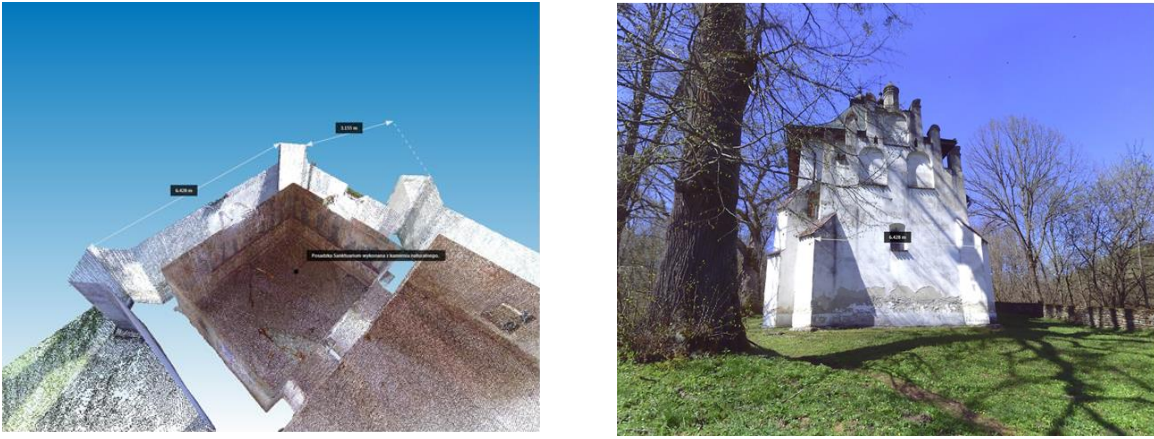
Figure 10. Example of dimensioning done in ReCap software
