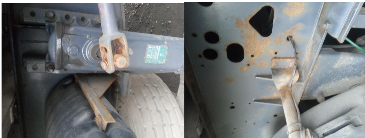
Fig. 1. An example of corrosion damage in elements of a heavy vehicle structure
