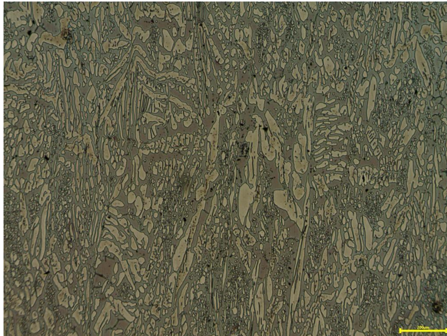
Fig. 6. A microstructure of the weld (B18)
