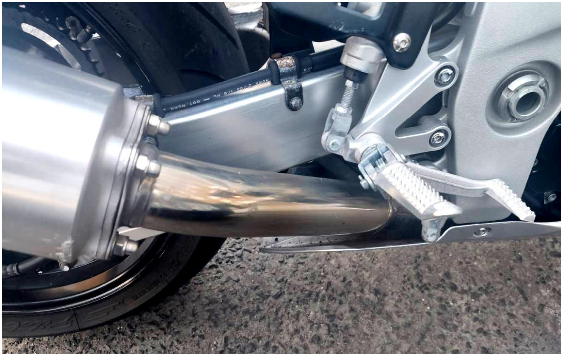
Fig. 2. Welded duplex steel elements in the motor vehicle
