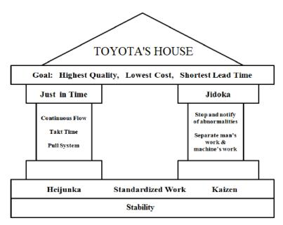
**Figure 2.** Toyota Production System. Toyota House. Source: Liker, 2005.
