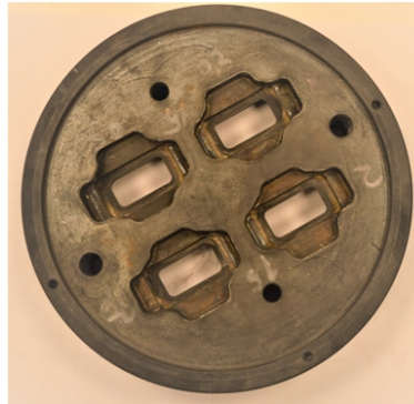
Figure 1: Extrusion die for aluminium alloy profiles [34].
