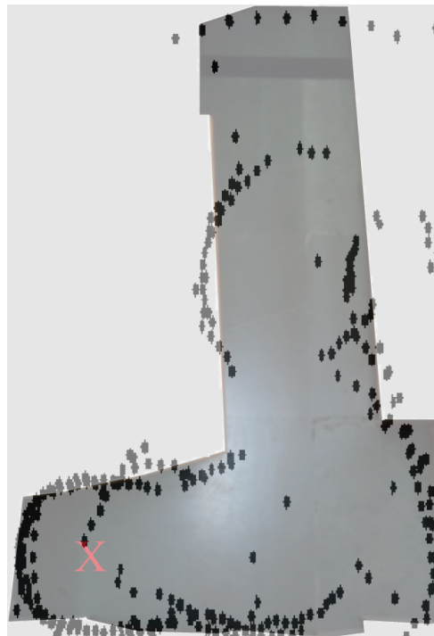
Fig. 9. Image of the room under consideration and the map created by the TriBot superimposed onto it
