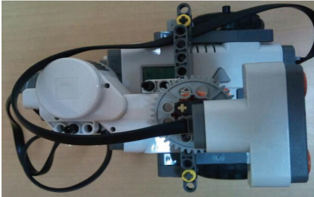
Fig. 1. Top view of the Lego Mindstorms NXT TriBot based robot with an interactive servo motor and the ultrasonic sensor attached on top
