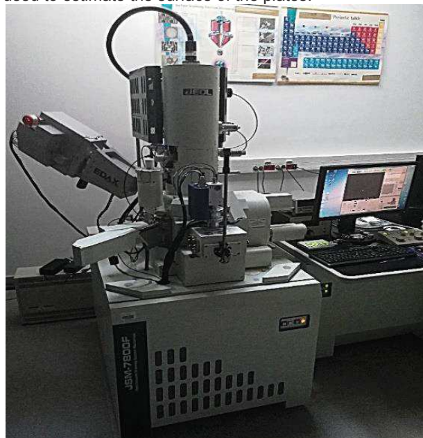
FIG. 2. Scanning electron microscope JSM-7800F.
