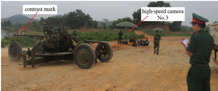
Fig. 10. Position of camera SA1.1 measures vertical displacement
