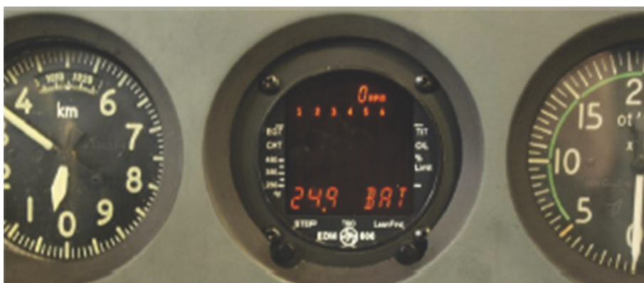
Figure 2. EDM-800's emplacement on the instrument panel in Zlin 43 [2]
