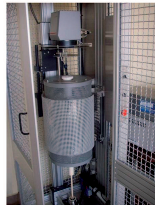
Fig. 2. Scheme of a high temperature rheometer FRS1600 [19-22]
