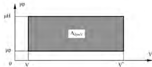
Fig. 6. Volumetric work A_{dyssV} as wear particles are generated in the system of coordinates shear stress – volume [L. 10]
