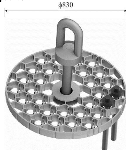
Fig. 2. Simple equipment used in a pit furnace for the heat treatment of long objects
