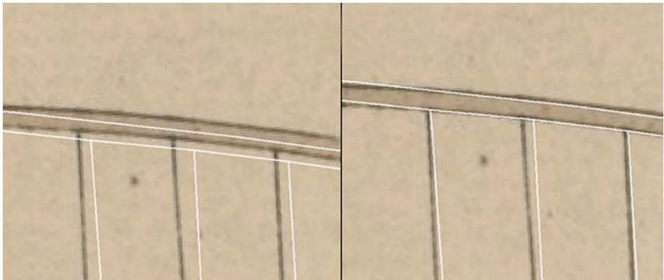
Fig. 3. Detailed calibration of the raster of the cadastral map by the affine transformation (left side – the state before, right side – after)
