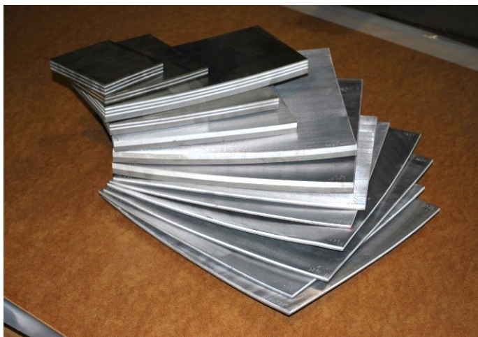
Figure 3. The batch of Ti6Al4V/AA2519 test plates
