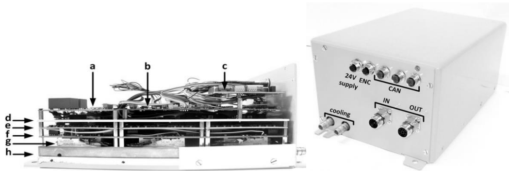
Fig. 0.4. Voltage source inverter for ECO-Car: a) DC voltages measurement board, b) control board with microcontrollers and FPGA unit, c) low voltage power supply board, d) mounting plate, e) IGBTs driver boards, f) DC-link board, g) IGBT modules, h) heat sink
