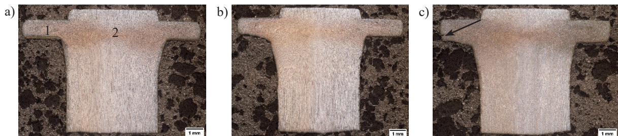
Fig. 6. Macrostructure of the cold-headed samples of wire rod of 32CrB4 steel after the following variants of cooling: a) variant W280; b) variant W395; c) variant W440. The average strain rate was 10^{-1}/\text{s}
