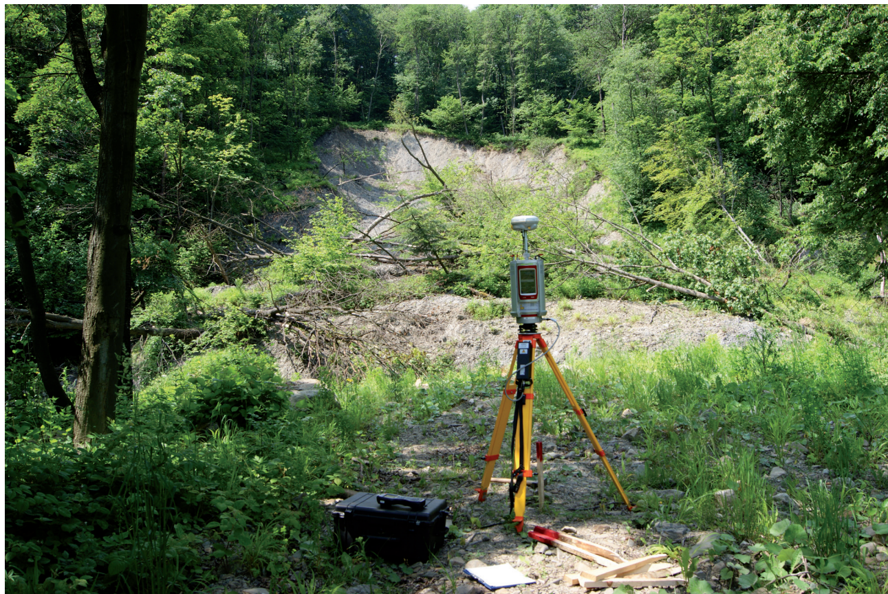
Ryc. 2. Skaner Riegl VZ 4000 na tle osuwiska Bodaki Fig. 2. Scanner Riegl VZ 4000 on a background of Bodaki landslide
