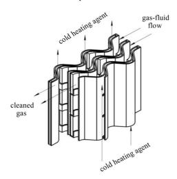
Fig. 1 Scheme of the flows moving during the inertial filtering process by condensation [*Sklabinskyy et al.*, 2014]
