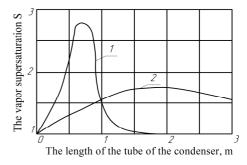
Fig. 2. Supersaturation along the length of the condenser pipes at various temperatures cooling water: 1-293 K, 2-313 K
