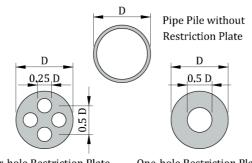
Four-hole Restriction PlateOne-hole Restriction PlateFig. 4. Restriction plates of various shapes that are mounted inside the pile foundation [9]
