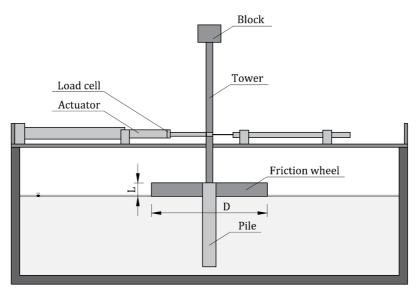
Fig. 6. Cross-sectional view of the analyzed hybrid pile model. The drawing was made on the basis of the article [12]
