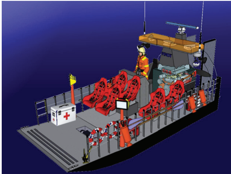
Fig. 1. One of the concepts of swimming flat-bottomed evacuation platform (Own develop of Automotive Industry Institute)
