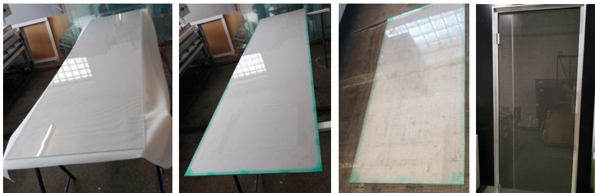
Fig. 9. Photos depicting the successive stages in the creation of the composite pane, in various size variants. Source: Photos from the collection of PIU Design
