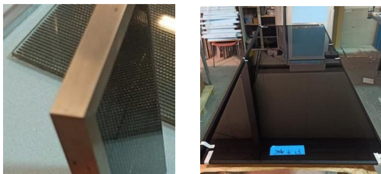
Fig. 10. Photos depicting the connections of the components of the border strip, which covers the edge in the version crimped at a 45-degree angle in the corner. Source: Photos from the collection of PIU Design
