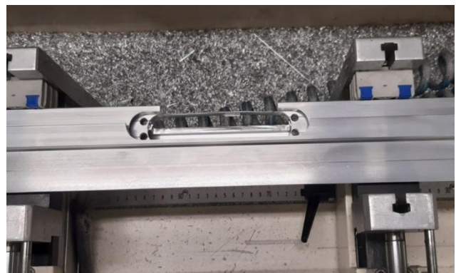
Fig. 17. Photos depicting the machining process of predefined locations for locks and hinges on a CNC machine for machining aluminium, the photos show the machining fixtures that position and clamp the profiles on the pneumatic clamps of the machine. Source: Photos from the collection of PIU Design
