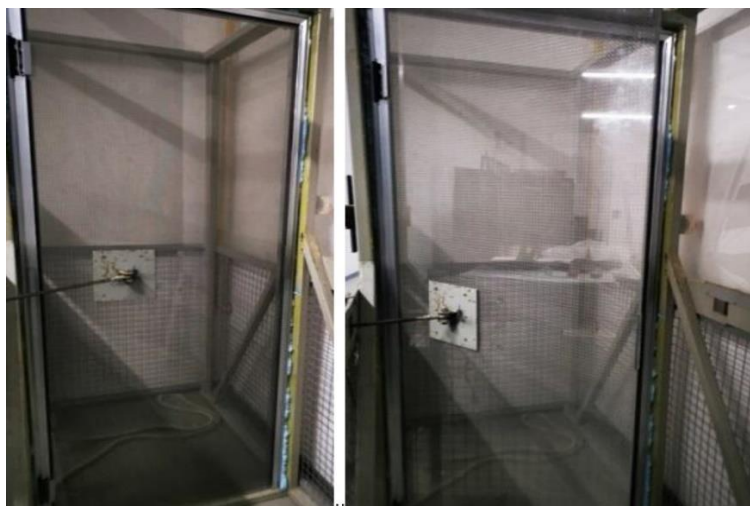
Fig.11. Photos depicting the PIU Glass door leaf on the test bench for testing repeated cyclic opening and closing. Source: Photos from the collection of PIU Design
