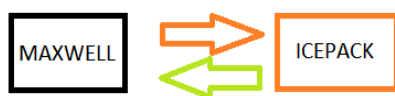
Fig. 3. "Coupling" diagram of the temperature calculation process (two separate programs calculate the temperature)
