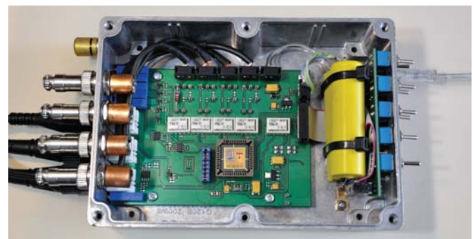
Fig. 10. Test setup for measurements of the readout IC (top cover removed)
