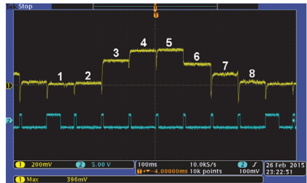
Fig. 6. Measurement of 8-pixel line, THz beam centered in-between the fourth and fifth pixels
