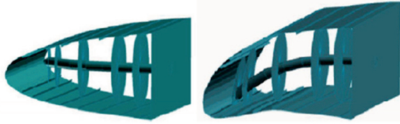
Fig. 2. The structural model of the wing in a standard position (left) and during deflection due to air pressure generated during flight (to the right) [4]
