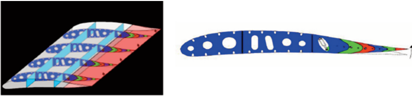
Fig. 5. Model of the elastic rear trailing edge of the wing [6]
