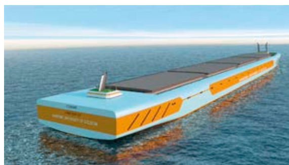
Figure 1. Visualisation of the design of an unmanned, autonomously controlled, container ship (bulk carrier) ( L_C = 78.75 m, B = 11.10 m, T = 4.33 m, \nabla = 2500 m 3 )
