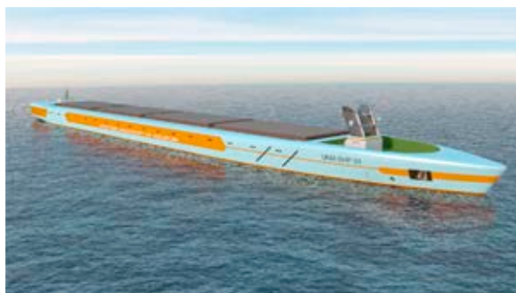
Figure 1. Visualisation of the design of an unmanned, autonomously controlled, container ship (bulk carrier) ( L_C = 78.75 m, B = 11.10 m, T = 4.33 m, \nabla = 2500 m 3 )
