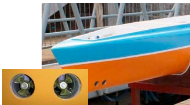
Figure 1. Visualisation of the design of an unmanned, autonomously controlled, container ship (bulk carrier) ( L_C = 78.75 m, B = 11.10 m, T = 4.33 m, \nabla = 2500 m 3 )
