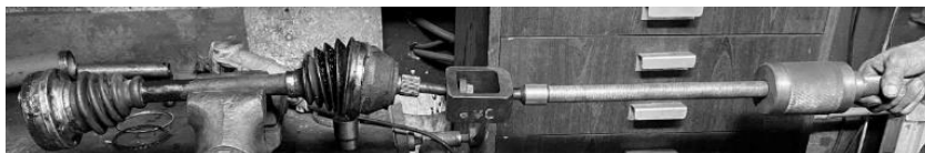
Fig. 2. The designed CV joint puller in its working position.
