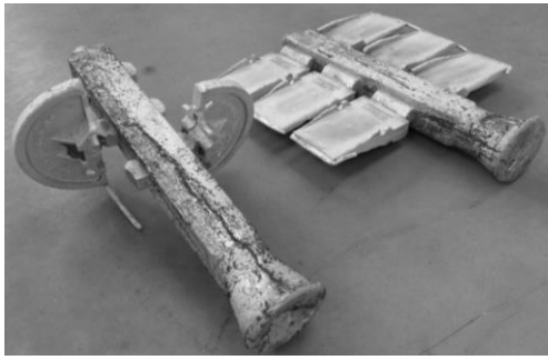
Fig.9. Castings made of magnesium AZ91 alloy in a mould made with the application of the new ceramic material.
