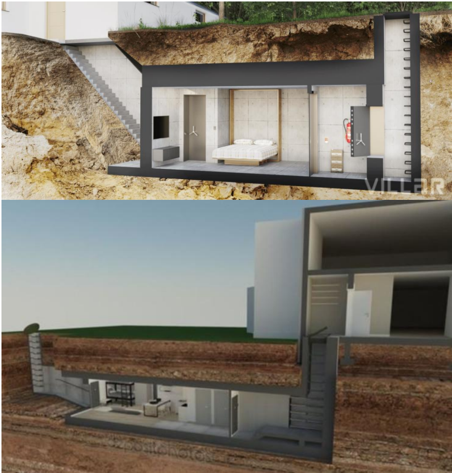
Fig. 9. Diagram of a family shelter in the basement or cellar of a building - the bidder did not provide parameters [23,24].
