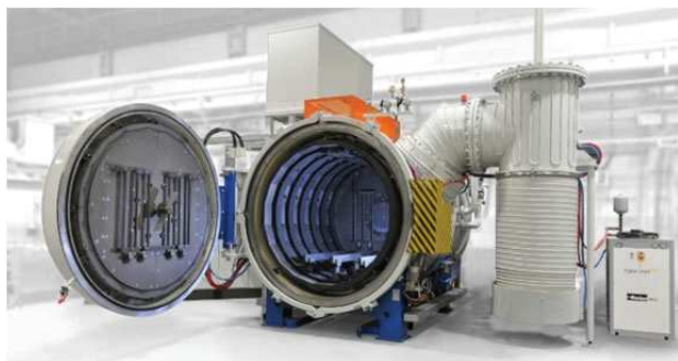
Fig. 7. High vacuum furnace with working zone 1200 x 1200 x 1800 mm
