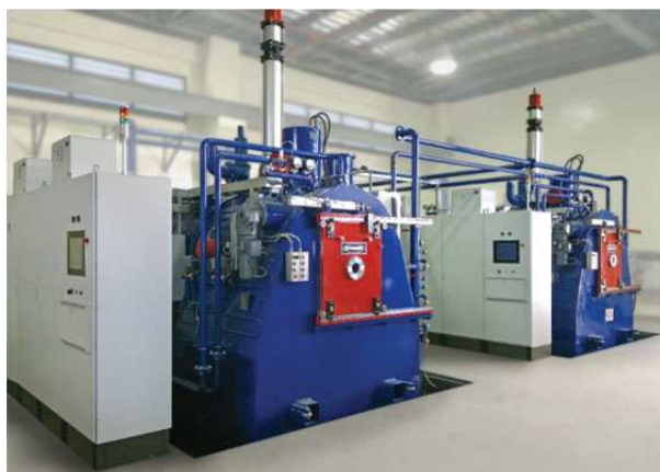
Fig. 1. The example of double chamber vacuum furnace
