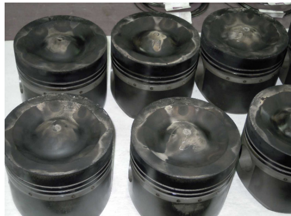
Fig. 14. View of pistons made of novel material after S12-U engine testing
