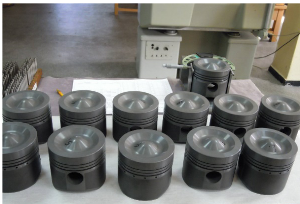
Fig. 3. The new pistons, made with new material, before S12-U engine installation
