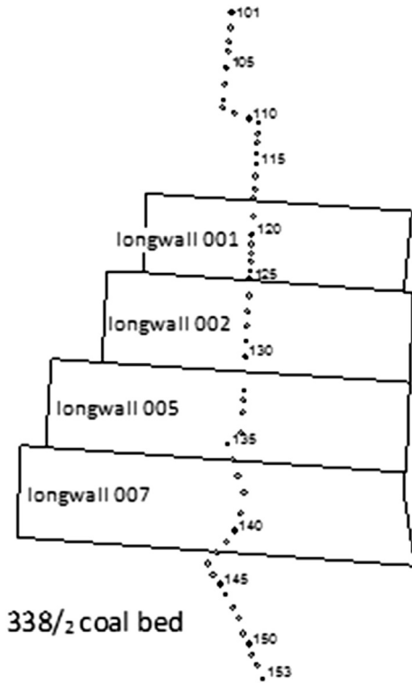
Fig. 2 – The location of a measuring line No. 1 in relation to the edges of longwalls 001, 002, 005 and 007, 338/2 coal bed.
