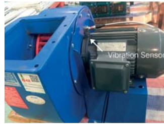
Fig. 2. Blower test bench
