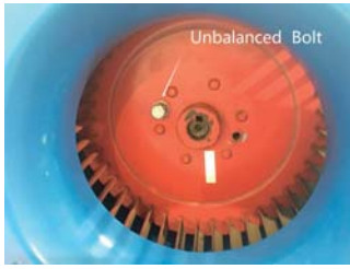
Fig. 1. Blower imbalance fault setting
