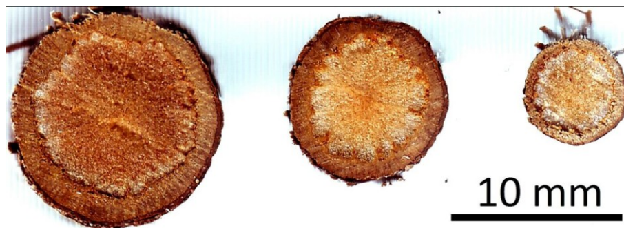
Figure 10. The pictures of cross-section of raspberry stalks (sponge tissue visible in the core zone) (source: own research).
