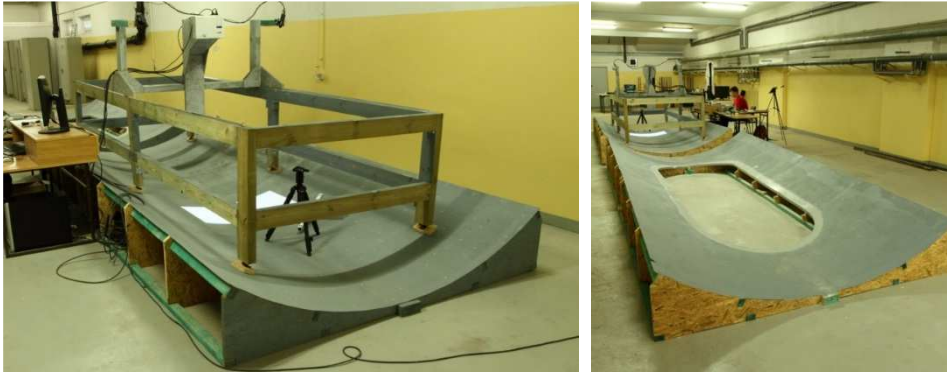
Fig. 1. Research stand and different models of steel plate with excised hole and edge simulation
