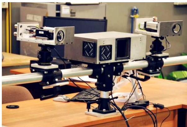
Fig. 10. Scanner head consists of two camera modules and projector module mounted on common beam
