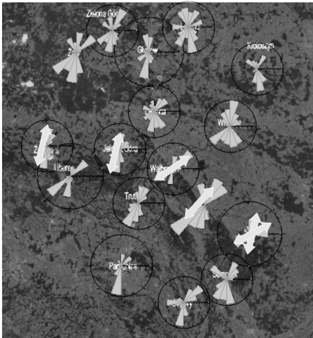
Fig. 12. Compilation of azimuth diagrams of over-represented daily displacements of all the stations. White arrows mark the azimuths of the stations situated nearby the Sudetes demonstrating their annular pattern.
