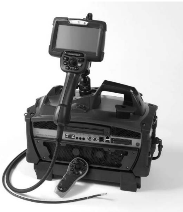
Figure 7. Video endoscope XLG3 Everest
