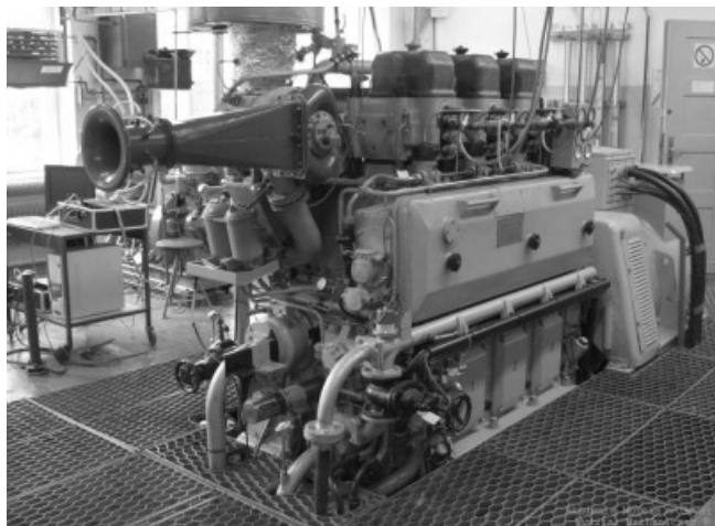
Figure 1. Marine diesel type 3AL 25/30
