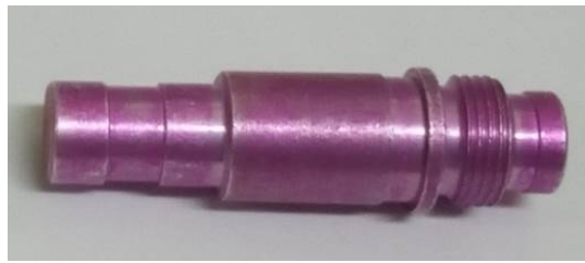
Photo 2. Pyrotechnic retarder of underwater rifle grenade NGP-76.
