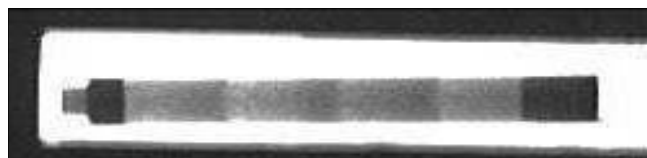
Photo 4. RTR photo of the NGP-76 underwater rifle grenade pyrotechnic retarder.
