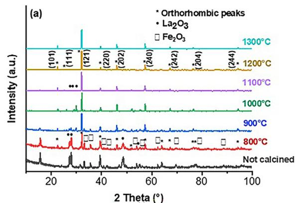
Fig. 2. X-ray diffraction patterns of LFO powders obtained at different calcination temperatures for a duration of 4 hours
