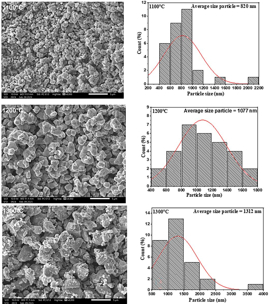
Fig. 5. SEM of the surface of LFO samples calcined at 1100°C, 1200°C, and 1300°C associated particle size distributions
