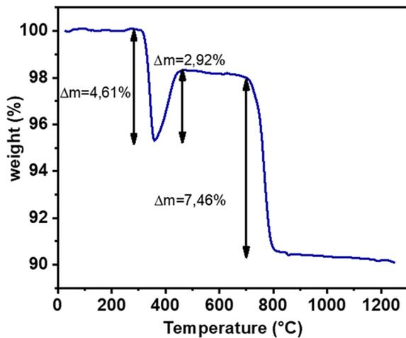
**Fig. 7.** Thermogravimetric analysis of LFO
