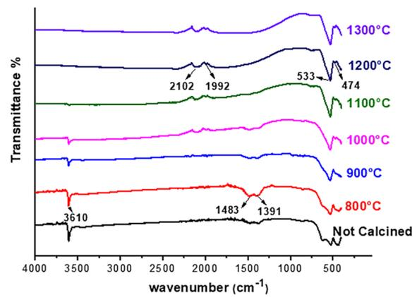
Fig. 4. FTIR spectra of the LFO samples at different calcination temperatures
