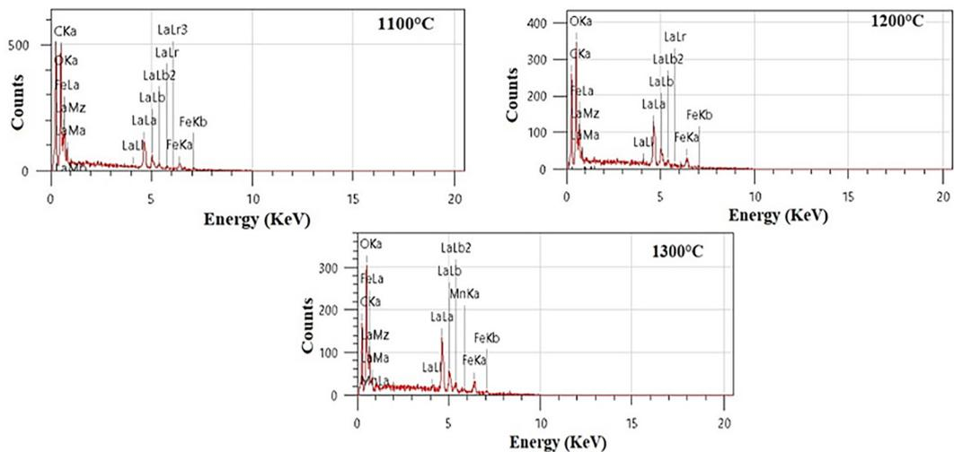
Fig. 6. Results of EDS analysis of LFO powders calcined at 1100°C, 1200°C and 1300°C for 4h
