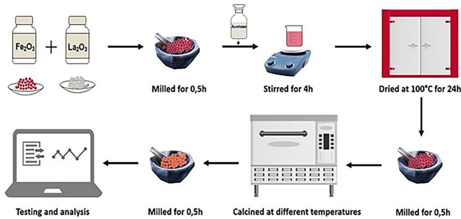
Fig. 1. Systematic synthesis procedure for LFO powders
