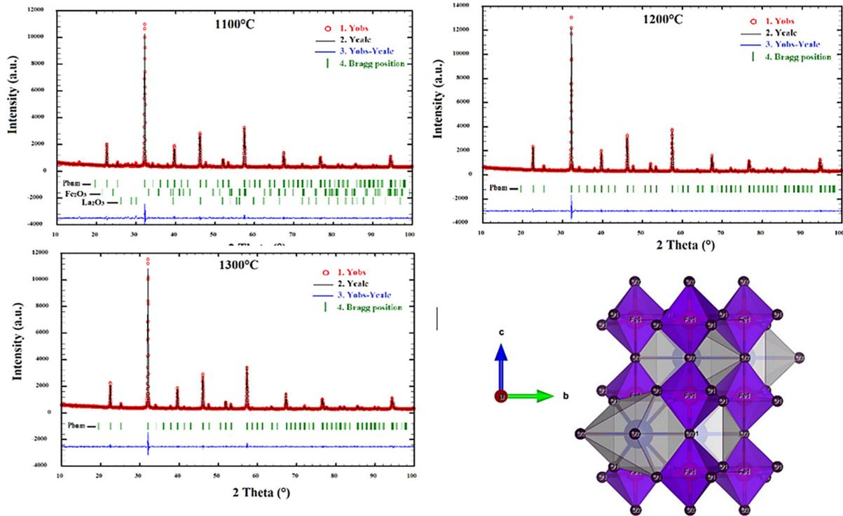
**Fig. 3.** Rietveld refinement for LFO calcined at 1100°C, 1200°C and 1300°C 4 h and the representation of polyhedral LFO calcined at 1200°C/4h obtained by the VESTA software
