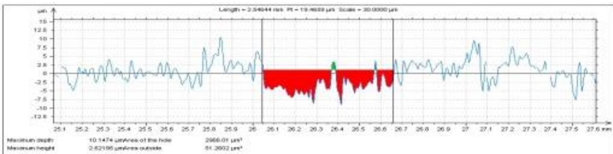
Fig. 4 Depth profile of coating 1350 wear trace
