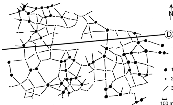
Fig. 5. The network of contraction cracks near Jasne Pole within the KKR area. Data based on Markuszewska (2006). D = road; 1 = circular depressions of over 50 m 2 ; 2 = circular depressions < 49 m 2 ; 3 = interpreted boundaries between the polygons.
