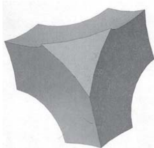
Fig. 2. Representative volume element of skeleton typical for carbon foams
