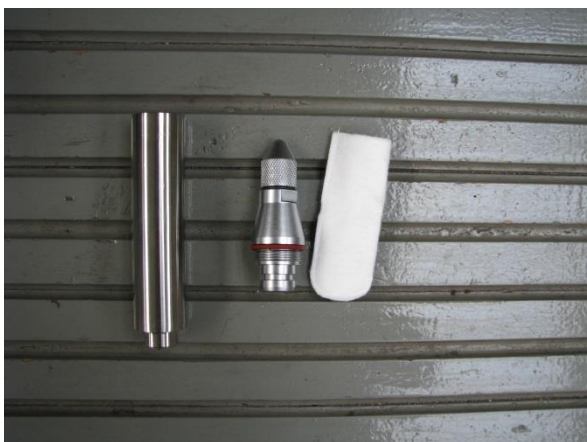
Fig. 2a. Separator and dust filter prepared for installation
