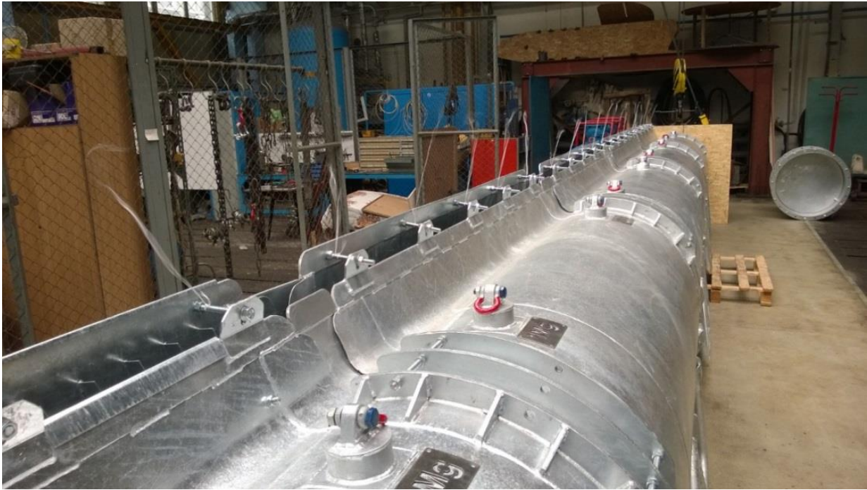
Fig. 6. Correctly adjusted vortex ventube
