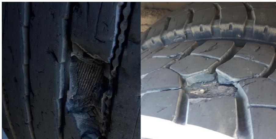
Fig. 19. An example of tearing off a tread fragment
