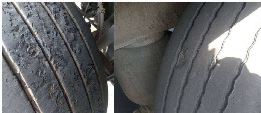
Fig. 17. Examples of cuts to the tread ribs
