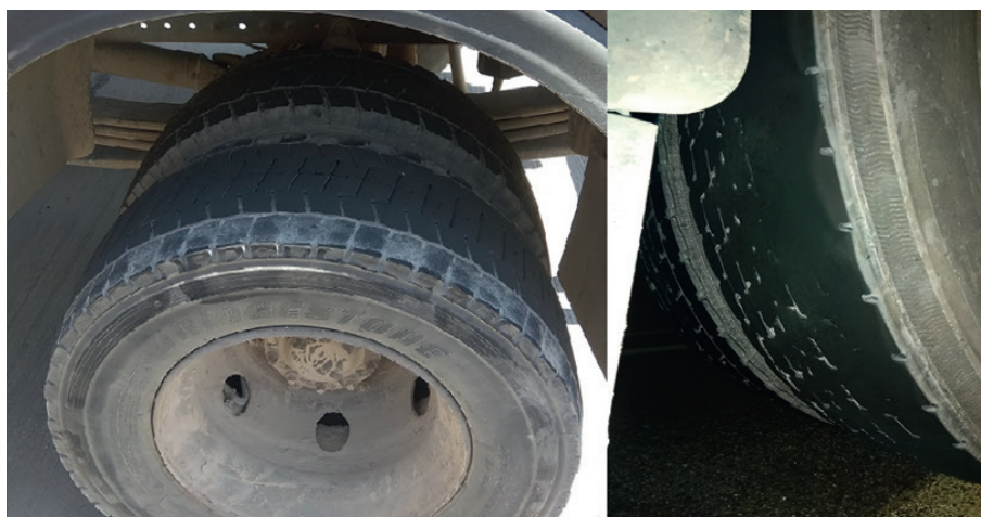
Fig. 24. Example of uneven tread wear
