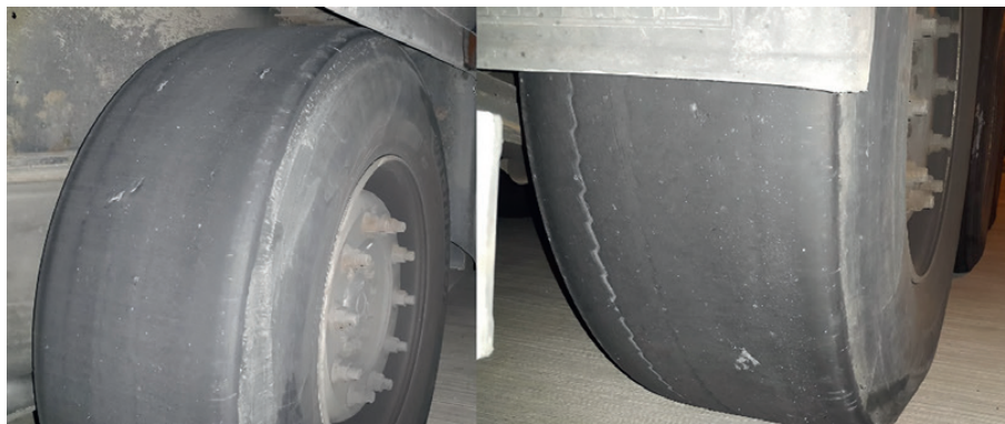
Fig. 22. Examples of emergency tread wear
