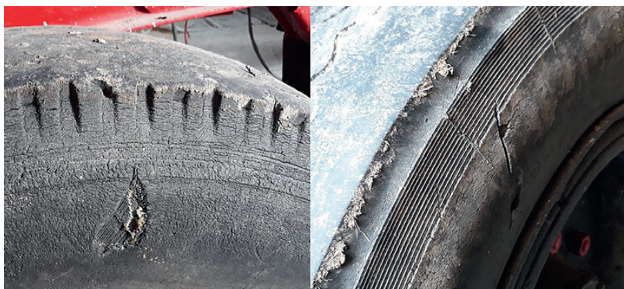
Fig. 18. Examples of tire sidewall damage
