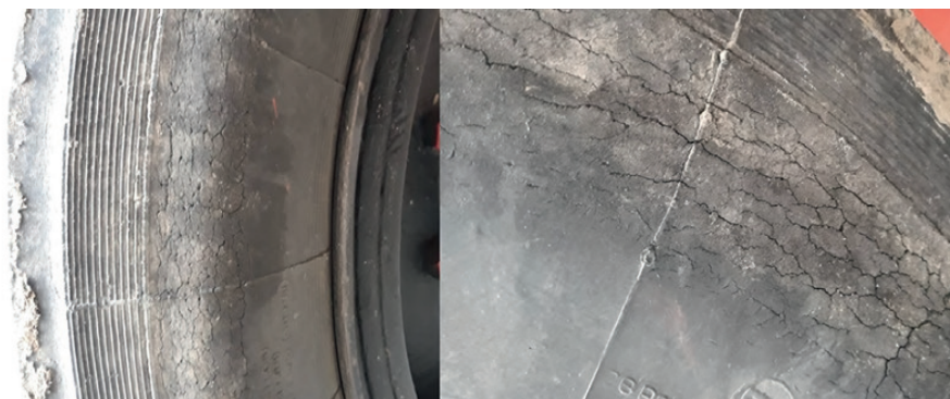
Fig. 21. An example of fatigue and aging cracks in a tire after long-term use
