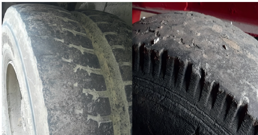
Fig. 23. Example of uneven tread wear
