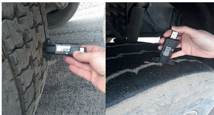
Fig. 2. Example of tire tread height measurements
