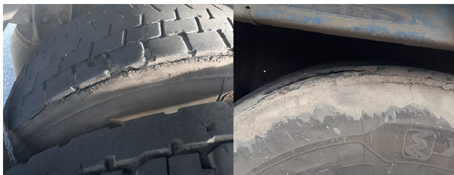
Fig. 20. Example of delamination of the tread layer
