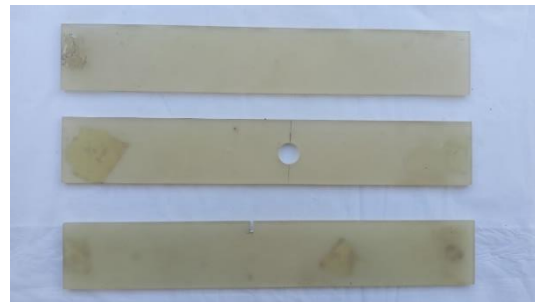
Fig. 1. The samples of the free vibration test
