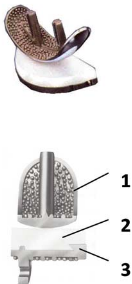
Figure 1. Knee joint endoprosthesis by W.LINK, 1 – metal sled, 2 – polyethylene UHMWPE insert, 3 – metal tibia part 20
