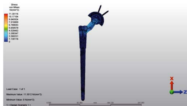
Figure 8. Distribution of stress in the analysed system at the load of 600N. Endoprosthesis head made of Ti6Al4V alloy
