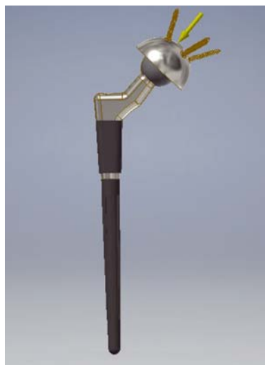
Figure 7. Surface where the loads were applied
