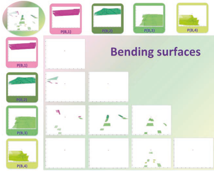
Figure 5. Bending surfaces of combination of sub-cluster-pairs. \mathbb{P}(B, k) represents a set of sub-cluster-pairs from bending clusters. For two \mathbb{P}(B, k) , it is possible to obtain corresponding combinations satisfying geometric constraints. Those sub-cluster-pairs that do not satisfy the geometric constraints will be eliminated, with no combinations for such two \mathbb{P}(B, k) , e.g., \mathbb{P}(B, 1) and \mathbb{P}(B, 4) .
