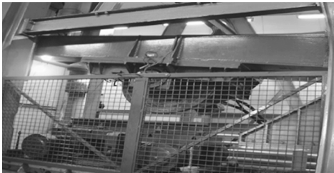
Fig. 2. Large-scale research station of the wheel-rail contact in the rolling-sliding contact [L. 2]
