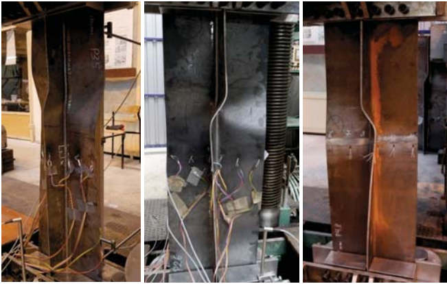
Fig. 10. Post-collapse shape for 5 mm (left), 6 mm (mid) and 8 mm (right) specimens
