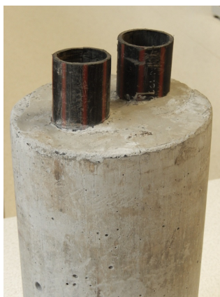
Fig 2. Model of the BHE cross-section with a single U-tube
