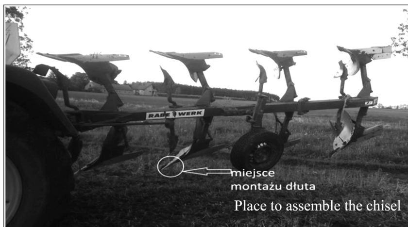
Fig. 1. Place to assemble the chisel [L. 8]
