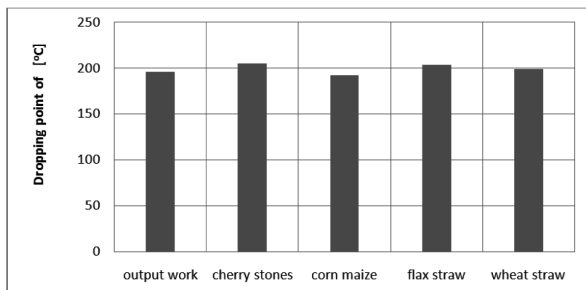
Fig. 13. The dropping point of biocarbon greases
