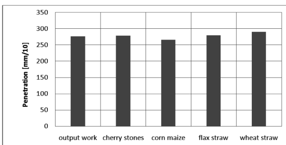
Fig. 14. The impact of biocarbon on the penetration of greases
